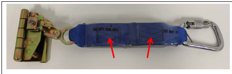
Cobra Rope grab shock absorber with two correct stitch patterns.
