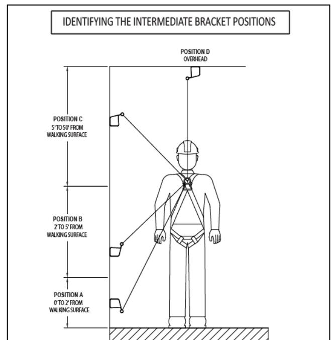
Although Capital Safety's testing shows the Sayflink Sleeve is safe to use in bracket positions B, C and D as illustrated above (and any height between these positions), out of an abundance of caution, Capital Safety is recalling all Sayflink Sleeves regardless of the height of the permanently installed brackets.
