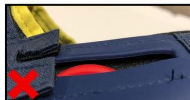
Step 2: Verify the rope length matches the unit specification as follows: Open the unit's backpack using the zipper on the back to locate the internal plastic bag that surrounds the spool and rope. If the plastic bag is missing, you have the incorrect length rope. If the bag is present and the rope fills half the spool, you have 50' rope. If the bag is present and the rope completely fills the spool, you have 100' rope.
