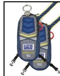
Step 1: Inspect to ensure the Assisted-Rescue Buddy Pull Ring (red ring below) is accessible from the outside of the unit. If not visible, reach into slot and pull the red ring handle out so that the flange going around the handle is secured between the two layers of material on the side of the bag containing the Pull Ring.
